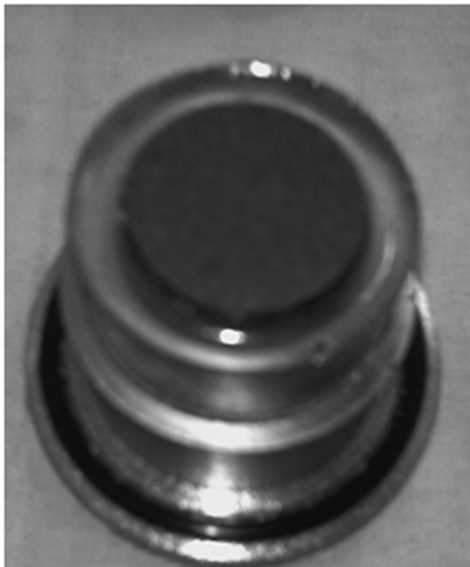
Fig. 6 Solid-propellant specimen of AP/Al propellant.
